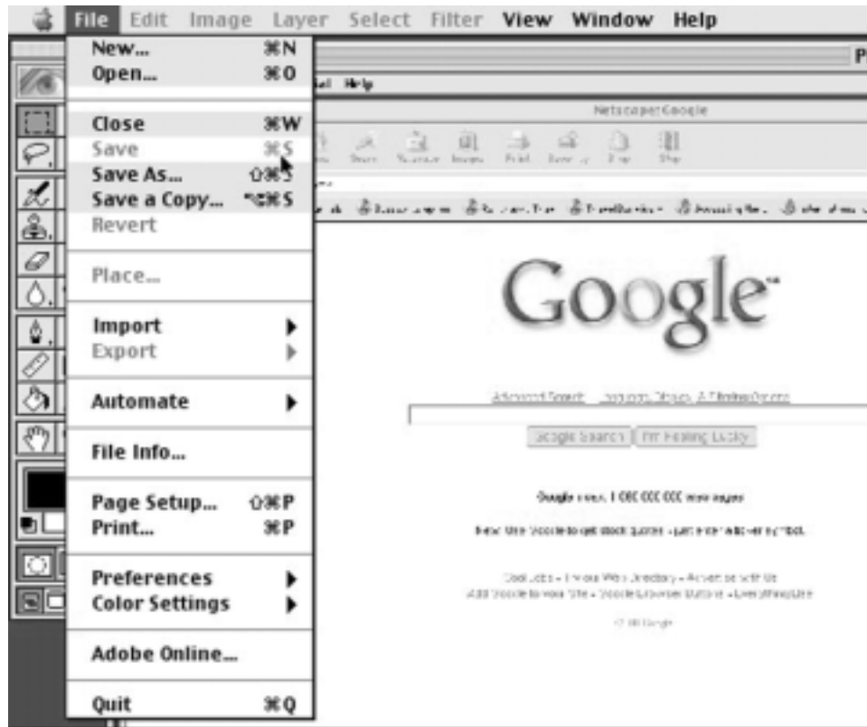
Figure 1.8 A menu illustrating restricted availability of options as an example of logical constraining. Shaded areas indicate deactivated options.
