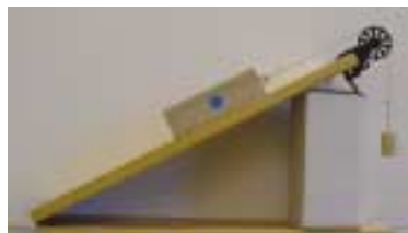
FIGURE 6-29 ■ Photograph of a block on an inclined plane that is moving at a constant velocity.
