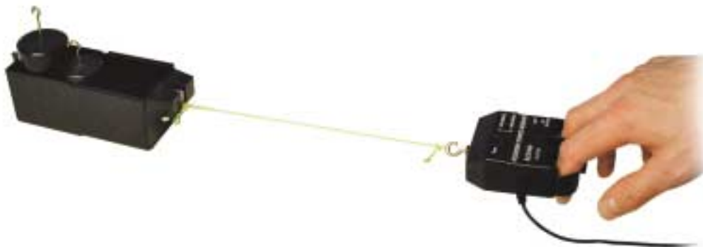
FIGURE 6-16 ■ The apparatus used for the static friction experiment includes an electronic force sensor attached to a computer data acquisition system (not pictured).
