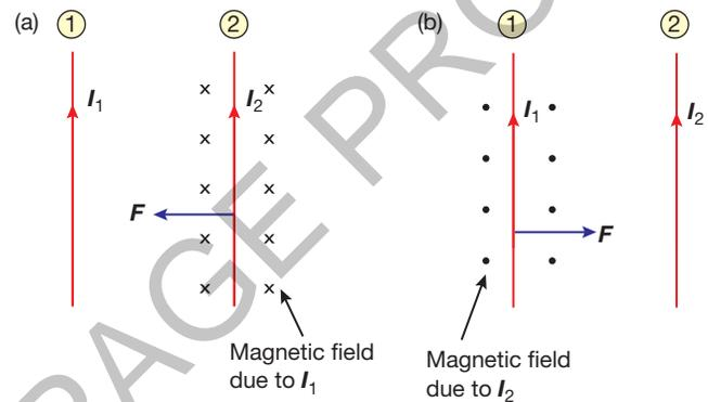
**FIGURE 5.15** The forces acting on two long parallel conductors carrying currents in opposite directions
