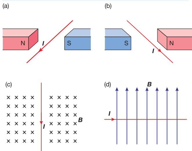
11. Deduce both the magnitude and direction of the forces acting on the lengths of conductors shown in figure 5.23.
