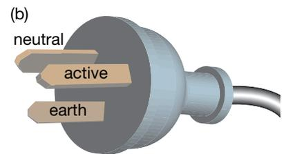
(a) A 3-point socket. The top left point is the active, the top right point is the neutral, and the bottom point is the earth connection. The switch is connected in the active wire. Also shown (b) is the wiring arrangement of a typical 3-point appliance plug. Note that the active pin is inserted into the active socket.
