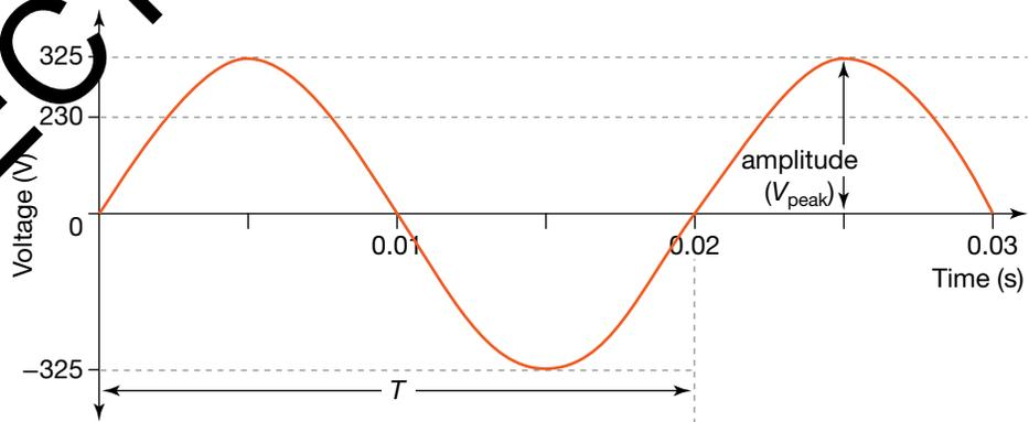
The variation of voltage with time for a supply of 230 V rms, 50 Hz.
