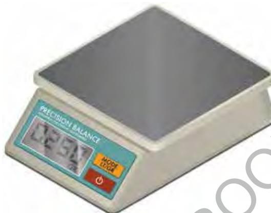
**Solution:** The scale shows 0.250 g, so the actual weight may be between 0.2495 g and 0.2505 g. The mass is written as  $0.250 \pm 0.0005$  g.
