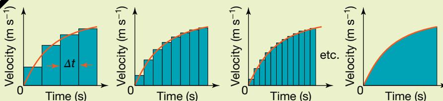
By dividing the velocity-versus-time graph into rectangles representing small time intervals, the displacement can be estimated.
